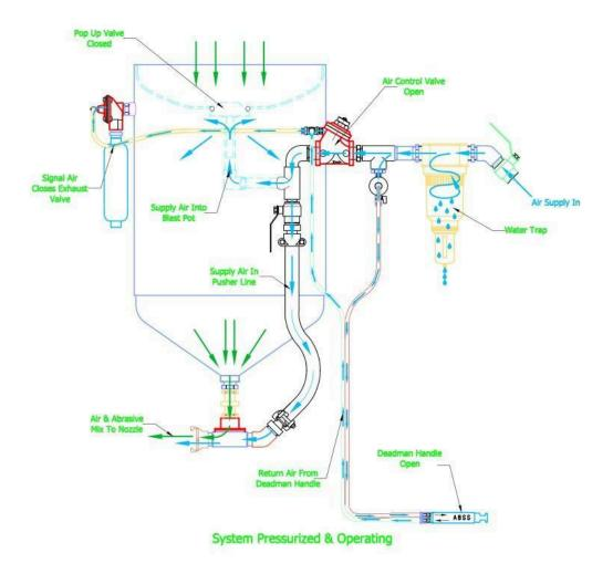
2.4 When the operator releases the deadman handle to stop blasting, the signal air to both the Air Control Valve and the Exhaust Valve is stopped, closing the Air Control Valve and opening the Exhaust Valve. This depressurises the pot, allowing the pop up valve to open, which in turn allows the pot to be refilled with abrasive media.
