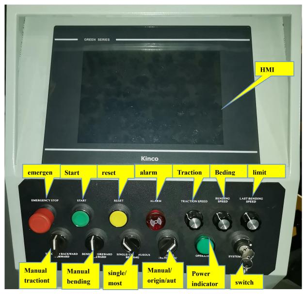
Note: The operation can only be performed after ensuring that the circuit is normal and the grounding wire is tight.
