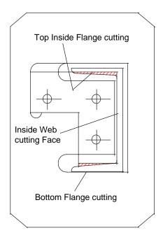
Fit blade to carrier, retain position with three screws, ensure blade is seating on both faces, see sketch. Mount a sample of channel, with a cleanly cut end, on to the blade with the bottom flange in line with bottom cutting face and the inside of the web square and in line with the inside web cutting face, as shown in sketch.
