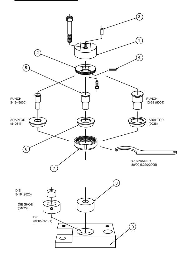
In the following table you can find a list of the standard punch tooling for a **Compact 40**. It includes equipment which is supplied as standard with the machine. The standard punch tooling includes an 18mm punch (9001) and die (9023). Other punches and dies are available on request.
