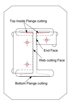
Fit blades to carrier, retain positions with fixing screws, ensure blades are seating correctly. Mount a sample of joist, with a cleanly cut end, on to the blade with the bottom flange in line with BOTTOM CUTTING FACE and the web square and in line with WEB CUTTING FACE, as shown in sketch.
