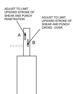
Stroke adjustement 'A' and 'B' can be adjusted by loosing the relevant actuator and sliding the actuator to the desired position.
