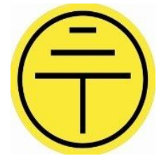
Hazard Earthing Point
