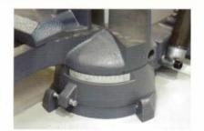
Large and well-readable angle scale helps to easily adjust the angle for mitering.
